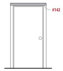
Length of rain drip should be the full width of the door frame.
